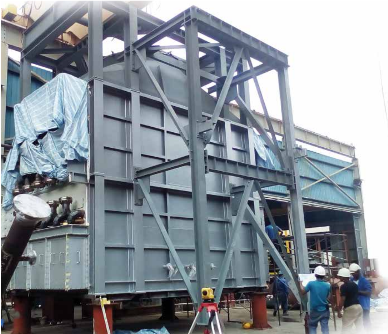
Fabrication & Assembly of Convection Modules & Transition, Gasco Abu Dhabi, U.A.E.
