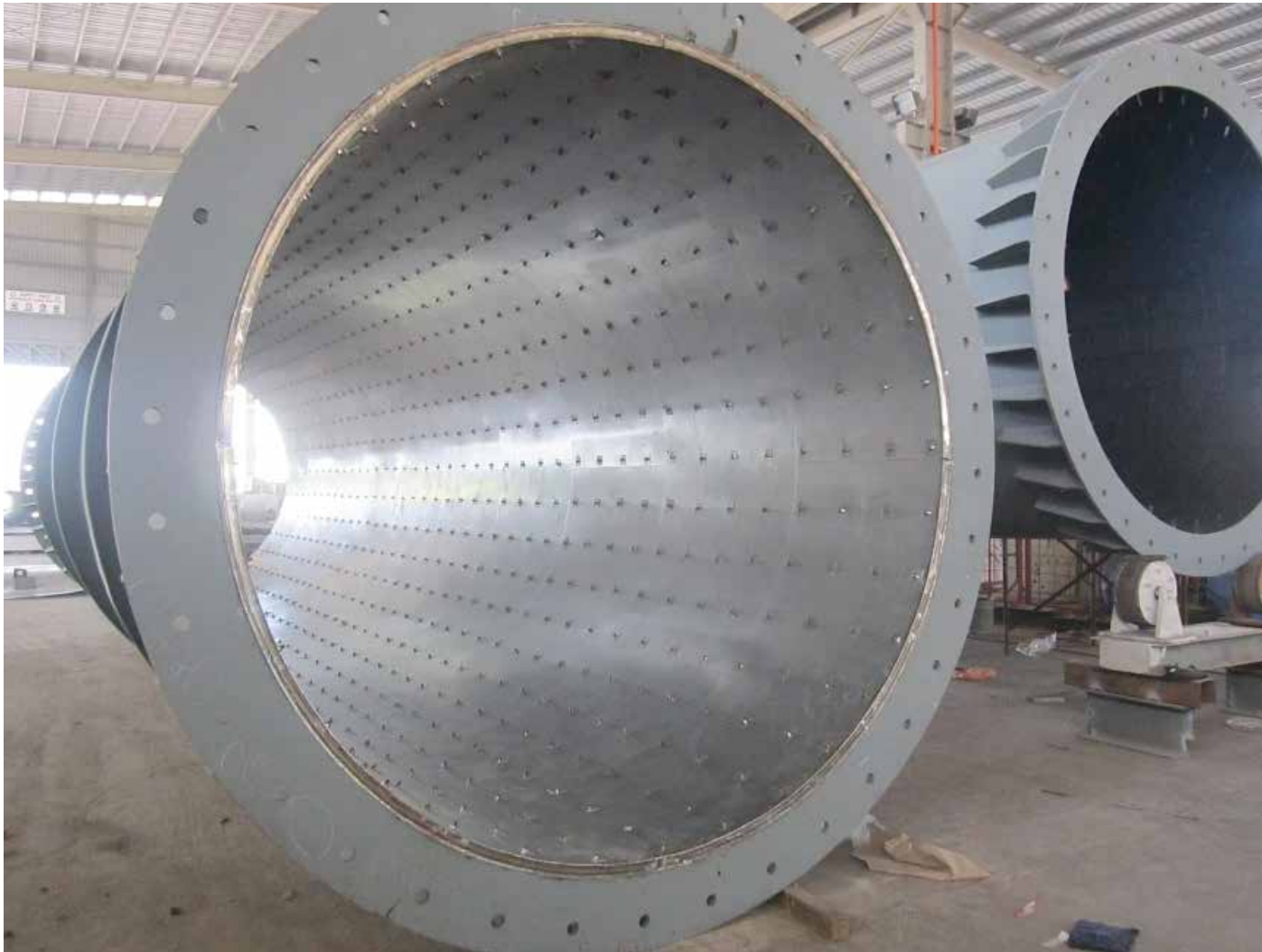
Fabrication GTG & GTC Stack & Duct with Structural Platforms, Petronas Floating LNG 2, South Korea
