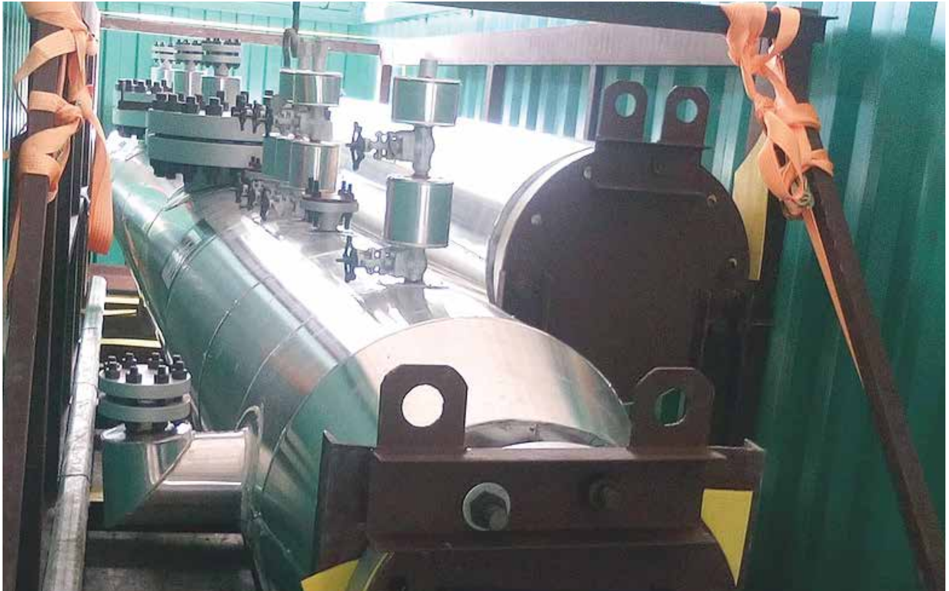
Main Steam Header with Piping, PT. Chandra Asri Petrochemical, Indonesia
